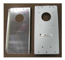
CNC-cut, Pre-punched, and formed from .032" 2024-T3 Aluminum. 2 per plane required. These are match drilled to the micarta ball assemblies. Included with Center Section kits. Available for \$9.50 each. (N/A with folding wing option)
