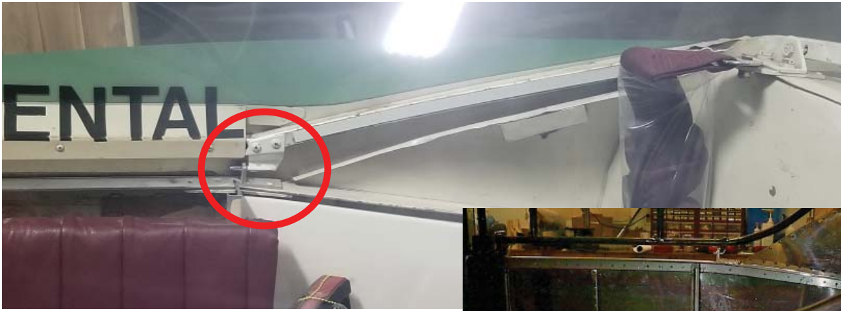
Aft Side Retaining Pins (p/n 280.386 & 387)
