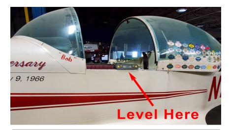
\*\* Note the tailwheel needs to be weighed in the level flight position. For a standard M-II, the cockpit side rails should be level as shown above.
