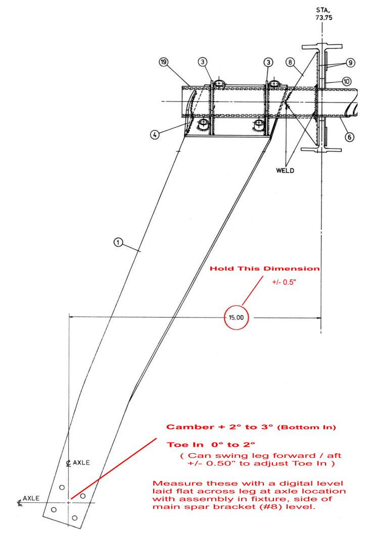
Weld Spacer to Spar Bracket
