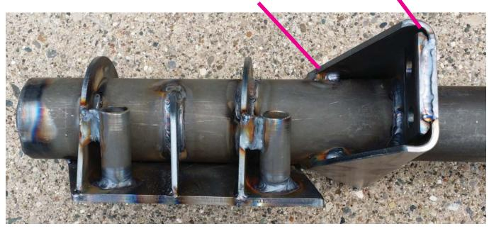
Weld Down Tube Inside Bracket 0.625" This is the CRITICAL Weld
